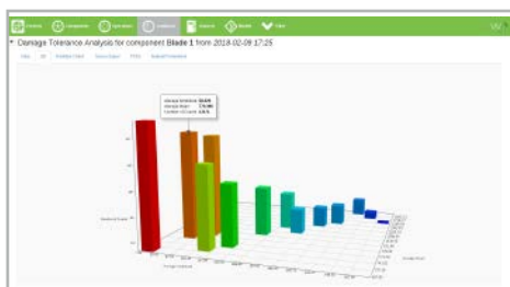
Damage tolerance analysis 3D histogram with load cycles
